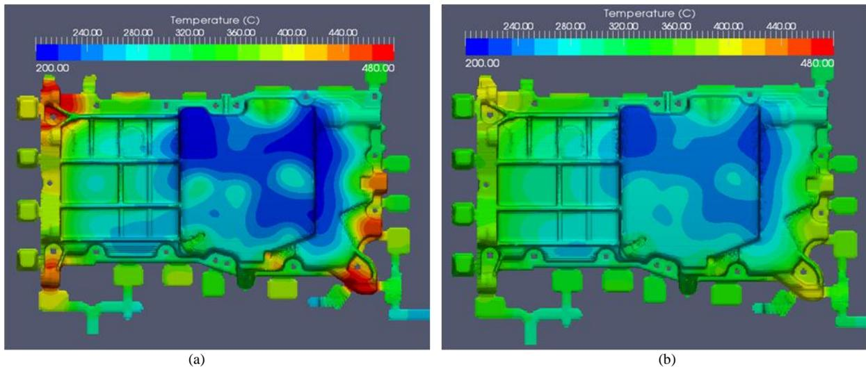
Fig.5. (a) Casting temperature before optimization, (b) Casting temperature after optimization
